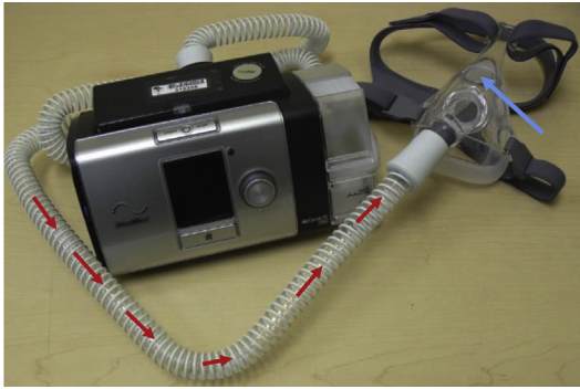
Fig. 1. In a single limb passive circuit, flow through the tubing is always in the direction of the patient as indicated by the red arrows . The blue arrow identifies the leak valve on the mask where excess flow and exhalation leave the circuit.
